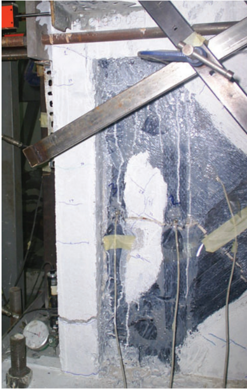
Figure 10 Damage state of specimen SA1.0-CV at 0.9% drift level.
