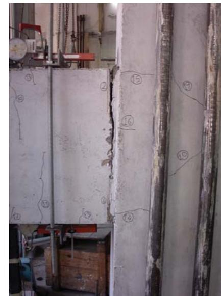
**Fig. 15.** Damage in specimen PTM50 at the 4% drift level.
