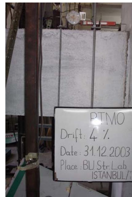
Fig. 9. Damage in specimen PTM0 at the 4% drift level.
