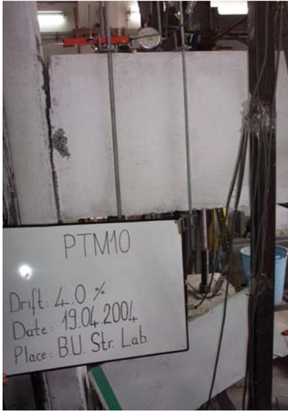
**Fig. 12.** Damage in specimen PTM10 at the 4% drift level.
