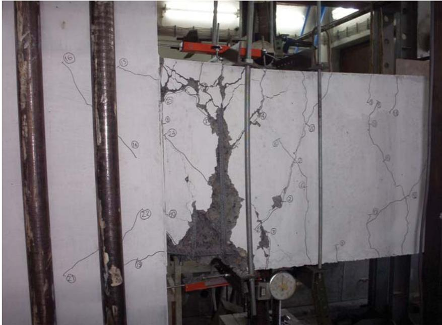
Fig. 7. Damage in monolithic specimen M at 4% drift level.
