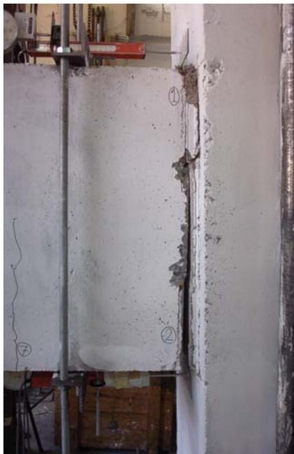
Fig. 17. Damage in specimen PTM65 at the 4% drift level.
